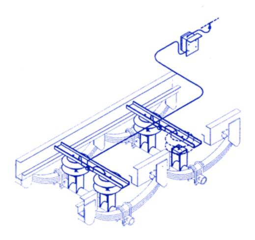
**Smooth Ride** is an add on air suspension system designed for most 96" or 102" wide single or tandem axle dry vans, reefers, or flatbed trailer installed with a spring suspension.
