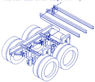
**Smooth Ride** has developed a new add on air suspension system designed to fit almost any trailer that currently has a spring suspension. While the idea of adding air bags to a spring suspension is not new, the **Smooth Ride** System is uniquely better and less costly.
